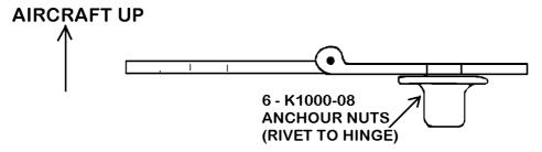
The next step is to install the four hinges in their proper positions on the top stabilizer skin. The anchor nut part of the hinge will go towards the elevator when actually installed. Place the hinges on the trailing edge of the upper skin with their pins centered over the recessed edge. Mark their hole locations. Check with a long straight edge to assure that all the hole marks fall on a straight line. If they do not the elevator will not hinge properly and the problem must be corrected.
