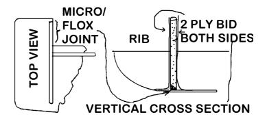
Before taking a break be sure to inspect the structure and all the glassed areas. The glass laminates should overhang the upper edges of the ribs and be in good contact with the rib sides, skin, and spar. If everything looks okay you can relax until its time for a green trim of the excess cloth hanging over the spar and ribs.
