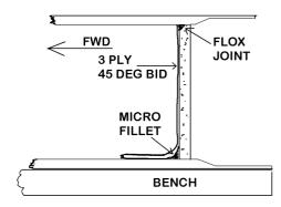
Also remove foam to form a flox slot at the top of each rib as shown. Fill the slot in the spar with flox. Pile the joint high with excess flox. Fill rib slots with flox; pile about ¼ inch of excess above the ribs. Carefully place the bottom skin in place as accurately as possible to avoid sliding. Use some strips of masking tape to hold the surfaces together and edges straight while the flox cures overnight.
