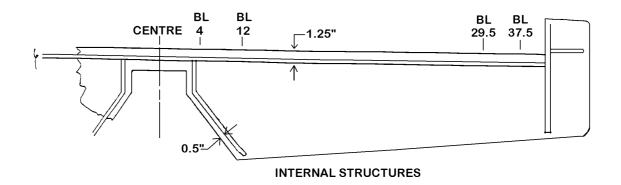
Prepare the top and bottom skins for subsequent layups by sandpapering the resin contact areas. These areas will be along the trailing edge bonding surface, within about 2 inches of both sides of the ribs, and from the hinge line aft about 3 inches. Also sand the entire inside area of the both skins in the right and left counterbalance areas. Mass balance weights will be bonded into these areas later.
