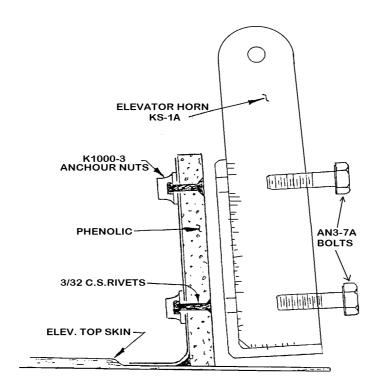
These nuts must be properly captured in position because once the bottom skin is in place they cannot be reached. Drill sixteen 3/32 holes through the spar from its forward face using an anchor nut as a drill guide. Countersink the holes slightly on the forward face so that countersunk type rivets can be used to secure the anchor nuts to the aft surface of the spar. Rivet the nuts in place using a rivet squeezer or small hammer to form the rivet heads.
