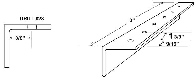
Use the angle bracket drill jig to locate and pilot drill the 12 holes in each hinge.
