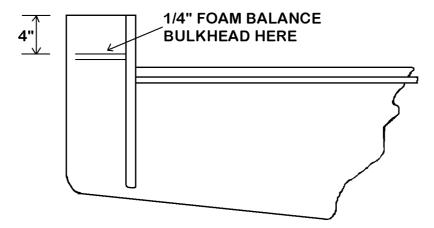
Before closing the assembly a pair of hinge spars must be installed for the single trim tab which will be on the starboard or right side of the aircraft. Mark its position as shown looking down on the inverted assembly.
