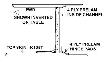
A "green" trim will be required to remove the excess BID along the 2 trailing edges of the channel. When completely cured block sand the edges to assure they are absolutely straight from tip to tip. This should help later when aligning hinges.
