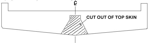
Handle the top skin with extreme care once the center cutout material is removed. It will be very easy to inadvertently damage the remaining glass in the center area.
