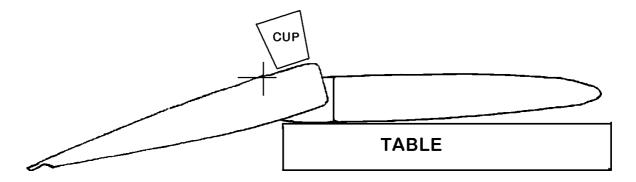
Mix the shot with some resin. Stir just a little flox into the mixture that results. Pour the mixture equally distributed into the left and right balance areas using the rib holes. Seal the rib holes with tape. Prop the horizontal tail so that the balances are down and the resined weight will cure in the very forward end of the balance structures.
