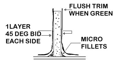
As with the spar corner, apply some micro to form small fillets at the bottom corners of the ribs. Then cut lengths from the 4 inch glass cloth strips and resin one layer of this cloth to each side of the six ribs. Once again the cloth should overlap the skin by about an inch. Make a flox joint as shown where the outboard sides of the outboard ribs interface with the skin. (Refer to Procedures Section for more on flox and micro/flox joints.) See drawing on next page.
