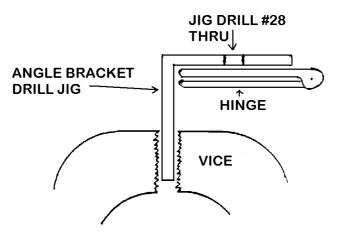
Accomplish this by clamping the angle in a vise. Close the hinge but space it slightly with some tape or thin cardboard. Clamp it in the closed or folded condition in the drill guide with one or two "C" clamps. Pilot drill the holes (two at a time) with a #28 drill bit. Drill all 14 hinges.
