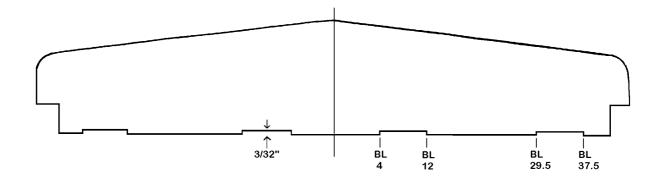
You will notice that the tip cavities are open. These should be faced with a piece of ¼ foam held in place with some 5-minute epoxy. After these are in place prepare the corners for flox joints, add the flox, and face the foam with one layer of BID.
