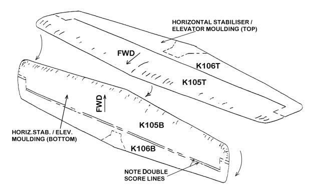
Find the scribe lines that will part the stabilizer and elevator on the outside of each molded piece. These lines run straight across and then around the elevator balance. Note that on the bottom piece only that there are two straight 81½ inch scribe lines rather than one. The ¾ inch piece in the middle gets removed to permit down elevator clearance when finished. Run a soft pencil along the lines for visibility.
