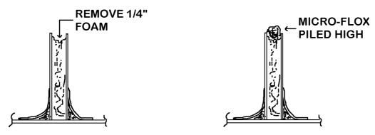
Prepare a 4-ply PreLam 7 inches wide for the open channel formed by the upper skin, lower skin, and spar. Run some micro/flox fillets along the corners and then squeegee the PreLam into place. Trim when ready.
