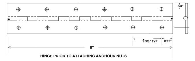
Make a precise drill jig from a scrap piece of aluminum or steel angle that has one leg about 1 inch wide. This guide will be used to make all 12 hinges on the aircraft so locate and drill the holes very accurately so that hinges are interchangeable and reversible.
