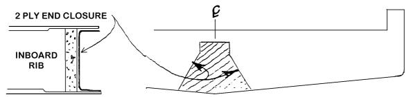
Once again install the elevator horn first making a ¾ inch relief slot in the bottom skin. Install all 8 bolts to assure clean fit.
